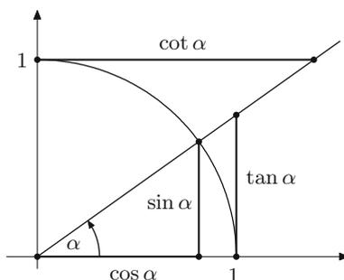
**Fig. 3.8** Extension of the trigonometric functions on the unit circle
