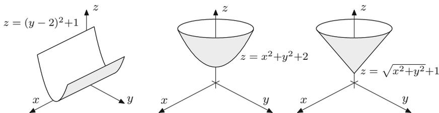
**Fig. 15.7** Local and isolated local minima. The function in the picture on the left has local minima along the straight line  $y = 2$ . The minima are not isolated. The function in the middle picture has an isolated minimum at  $(x, y) = (0, 0)$ . This minimum is even a global minimum. Finally, the function in the picture on the right-hand side has also an isolated minimum at  $(x, y) = (0, 0)$ . However, the function is not differentiable at that point
