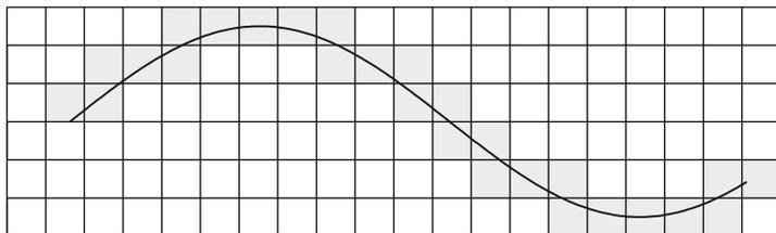
**Fig. 9.3** Raster of the plane using squares of side length  $\varepsilon$ . The boxes that have a non-empty intersection with the fractal are coloured in grey. In the picture we have  $N(A, \varepsilon) = 27$
