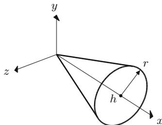
**Example 11.16** (Volume of a cone) The rotation of the straight line  $y = \frac{r}{h}x$  around the  $x$ -axis produces a cone of radius  $r$  and height  $h$  (Fig. 11.6). Its volume is given by
