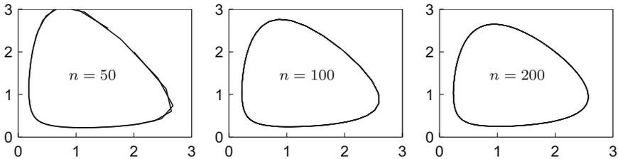
**Fig. 21.6** Numerical computation of a periodic orbit of the Lotka–Volterra model. The system was integrated on the interval  $0 \leq t \leq 14$  with the modified Euler method with constant step sizes  $h = 14/n$  for  $n = 50, 100$  and  $200$
