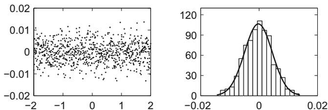
**Fig. 7.6** The left picture shows random noise which masks the data. The noise is modelled by 801 normally distributed random numbers. The frequencies of the chosen random numbers can be seen in the histogram in the right picture. For comparison, the (scaled) density of the corresponding normal distribution is given there as well
