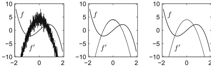
**Fig. 7.7** Numerically obtained derivative of a noisy function  $f$ , consisting of 801 data values (left); derivative of the same function after filtering using a Gaussian filter (middle) and after smoothing using splines (right)
