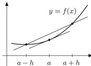
with  $|\varepsilon| \leq \text{eps}$ . The rounding error turns out to be proportional to  $\text{eps}/h$  and increases dramatically for small  $h$ . This behaviour can be seen in the numerical experiment for  $h$  between  $10^{-8}$  and  $10^{-16}$ .
